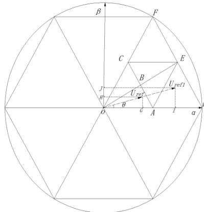
Figure 3 Three-level space voltage vector diagram
