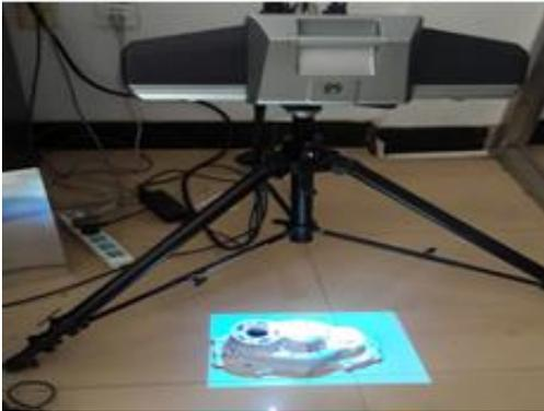
Fig. 4. The measurement system based on structured light
