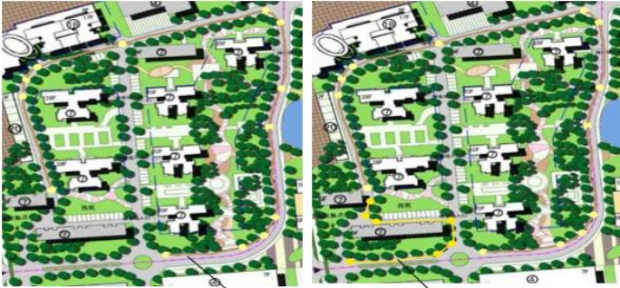
Existing path Add path Fig 6: Example of generating a new cable path
