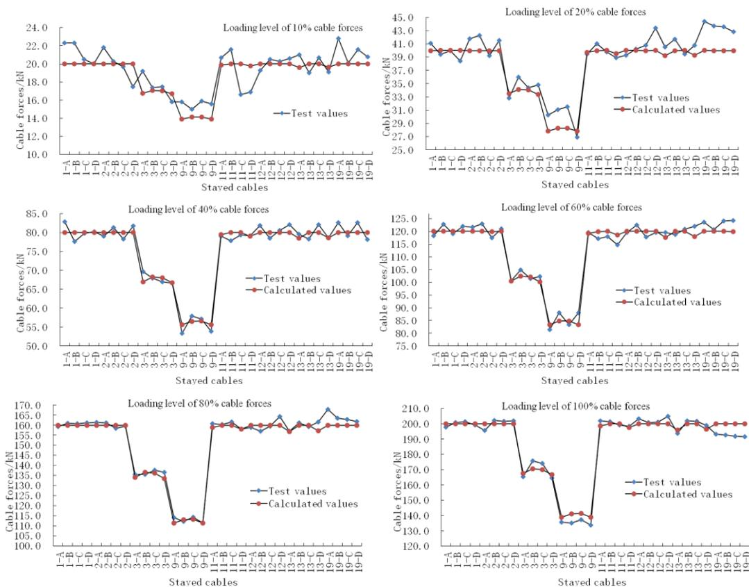
Fig 7: Calculated cable forces and test cable forces at each load level under case II
