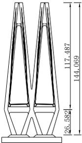
Fig 2: Elevation drawing of the bridge pylon/m
