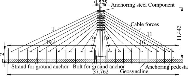
Fig 3: Elevation drawing of the model /m
