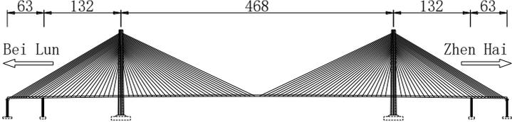
Fig 1: Elevation drawing of Yongjiang super-large bridge /m
