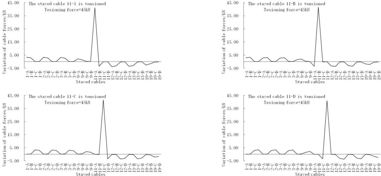
Fig 8: Variation of all cable forces when some cables are tensioned at the 100% load level under case II
