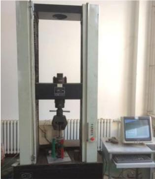
Fig 4: Single-hole compression molding test device for peanut straw
