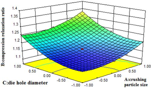
Fig 7: Response surface chart of die hole diameter crushing particle size and compression relaxation ratio
