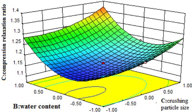
Fig 5: Response surface chart on water content crushing particle size and compression relaxation ratio
