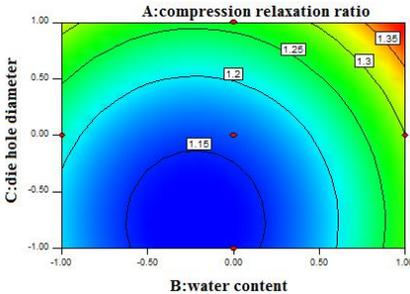
Fig 10: Contour map of moisture content die hole diameter and compression relaxation ratio
