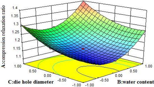
Fig 9: Response surface chart of water content die hole diameter and compression relaxation ratio
