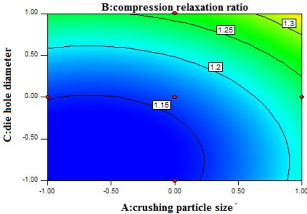
Fig 8: Contour map of die hole diameter crushing particle size and compression relaxation ratio
