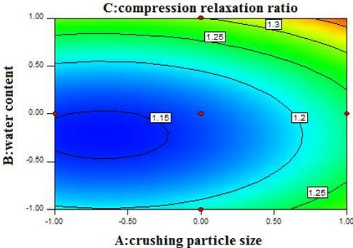
Fig 6: Contour map of moisture content crushing particle size and compression relaxation ratio
